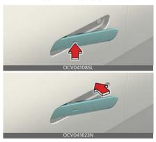
When all doors are closed, touch the touch sensor on the front outside door handle (the engraved part) while carrying the smart key with you, outside door handle will return and doors will be locked.
