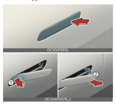
Push the button on the front outside door handle (the engraved part) while carrying the Smart Key with you, all doors will unlock.
