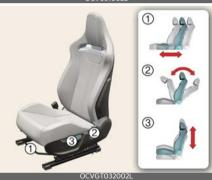
The front seat can be adjusted by using the control levers located on the outside of the seat cushion.
