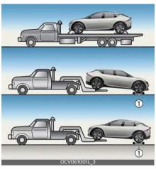
Proper lifting and towing procedures are necessary to prevent damage to the vehicle. The use of wheel dollies (1) or flatbed is recommended.
