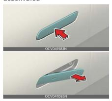
The handle does not slide out even when you approach with the smart key in possession. The doors are unlocked if you press the outside handle as the handles slide out.
