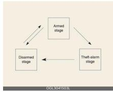
This system is operated in three stages: the first is the "Armed" stage, the second is the "Theft-alarm" stage, and the third is the "Disarmed" stage. If triggered, the system provides an audible alarm with blinking of the hazard warning lights.
