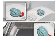
The devices should draw less than 10 amps with the vehicle on.
