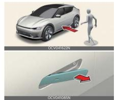
If you approach (within 30 cm (1 ft.)) the driver or front passenger's door handle possessing the smart key, the outside door handles slide out and the doors are unlocked. In this case, Hazard Warning
