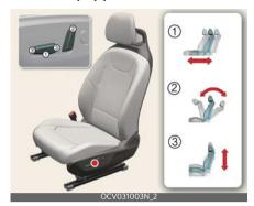
The front seat can be adjusted by using the control switches located on the outside of the seat cushion.
