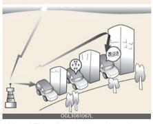
AM and FM radio signals are broadcast from transmitter towers located around your city. They are intercepted by the radio antenna on your vehicle. This sig-
