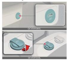
The electrical devices can be recharged when the vehicle is in ACC/ON position. The battery charging state may be monitored on the electrical device.
