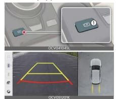
360° camera monitoring system can assist in parking by allowing the driver to see around the vehicle.
