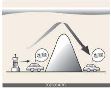
AM broadcasts can be received at greater distances than FM broadcasts. This is because AM radio waves are transmitted at low frequencies. These long distance, low frequency radio waves can follow the curvature of the earth rather than traveling straight. In addition, they curve around obstructions resulting in better signal coverage.
