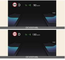
If the speed limit of the road changes during the operation of Manual Speed Limit Assist or Smart Cruise Control, an arrow in the direction of up or down is displayed to inform the driver that the set speed needs to be changed. At this
