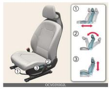
The front seat can be adjusted by using the control levers located on the outside of the seat cushion.
