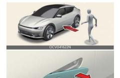
If you approach (within 30 cm (1 ft.)) the driver or front passenger's door handle possessing the smart key, the outside door handles slide out and the doors are unlocked. In this case, Hazard Warning Flasher blinks twice and chime also sounds twice.
