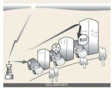
AM and FM radio signals are broadcast from transmitter towers located around your city. They are intercepted by the radio antenna on your vehicle. This sigFeatures of your vehicle Audio system
