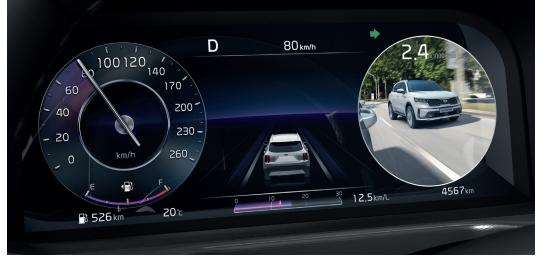
**Blind-view monitor**<sup>1,2</sup> activates within the instrument panel when you turn on the blinker to change lanes, to display the blind spot in the direction of your turn signal.
