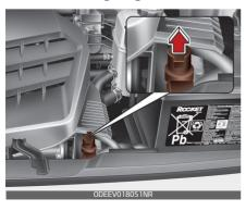
If the charging connector does not disconnect due to battery discharge and/or failure of the electric system, open the hood and slightly pull the emergency cable. The charging connector will then disconnect.
