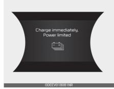
When the high voltage battery level reaches around 3% or less, this warning message is displayed.
