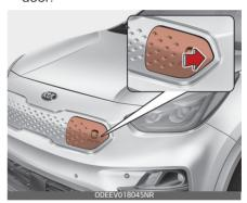
You cannot open the charging door when the vehicle's doors are locked.
