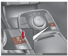
Push the button to turn off the Reverse Parking Distance Warning system. The indicator light on the button will turn on.
