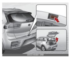
Only the liftgate is unlocked if the liftgate unlock button on the smart key is pressed for approximately 1 second.
