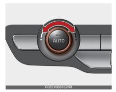
The temperature will increase to the maximum (28 °C) by turning the knob to the extreme right.
