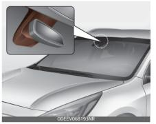
The auto defogging system operates when the heater or air conditioning is on.
