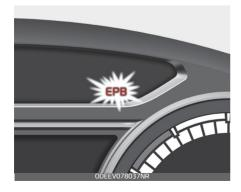
If the EPB malfunction indicator remains on, comes on while driving, or does not come on when the POWER button is changed to the ON position, this indicates that the EPB mau have malfunctioned.
