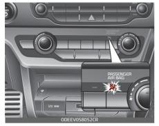
The occupant detection system is designed to detect the presence of a properly-seated front passenger and determine if the passenger's front air bag should be enabled (may inflate) or not. Only the front passenger front air bag is controlled by the Occupant Detection System.
