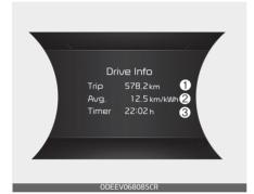
This display shows the trip distance (1), the average energy consumption (2), and the total driving time (3).
