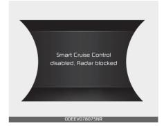
When the sensor cover is blocked with dirt, snow, or debris, Smart Cruise Control system operation may stop temporarily. If this occurs, a warning message will appear on the LCD display. Remove any dirt, snow, or debris and clean the radar sensor cover before operating Smart Cruise Control system. Smart Cruise Control system may not properly activate, if the radar is totally contaminated, or if any substance is not detected after turning ON the vehicle (e.g. in an open terrain).
