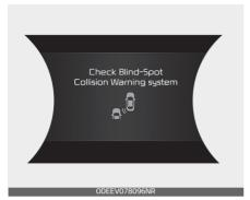
If there is a problem with the BCW system, a warning message will appear and the light on the button will turn off. The system will turn off automatically. RCCW will not operate also if BCW system turns off due to malfunction. Have your vehicle inspected by an authorized Kia dealer.
