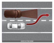
When a vehicle changes lanes in front of you, the smart regeneration system may not immediately detect the vehicle, especially if the vehicle changes lanes abruptly. In this case, you must maintain a safe braking distance, and if necessary, depress the brake pedal to reduce your driving speed in order to maintain a safe distance.
