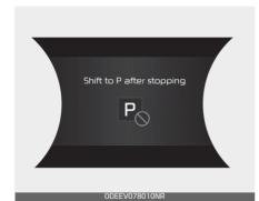
The message appears on the LCD display when the gear is shifted to P (Park) while the vehicle is moving.
