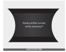
The message appears on the LCD display when the shift dial is not turned while pressing P button.
