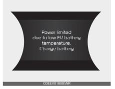
The warning message is displayed to protect the electric vehicle system when you turn off or turn on the vehicle while outside temperature is low. If the high voltage battery charging level is low and parked outside in low temperature for a long time, vehicle power could be limited. Charging the battery before driving, increases the battery temperature, and helps increase power.
