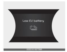
When the high voltage battery level reaches around 8% or less, this warning message is displayed.
