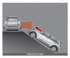
The system may not operate properly when the vehicle is on/near a slope.
