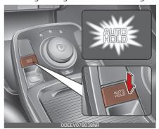
Before the Auto Hold will engage, the driver's door and vehicle hood must be closed and the liftgate must be closed.
