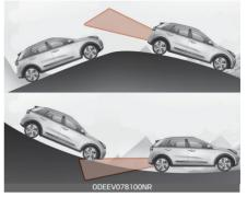
BCW systems may not operate properly when driving on a slope. In certain instances the system may not detect the vehicle in the next lane.
