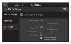
You can apply electric car-related functions for guiding the route. It allows you to check the distance
