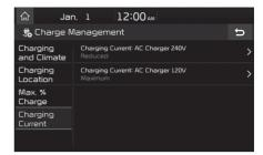
If the charging process does not start or abruptly stops in the middle, re-select another proper current and retry charging the vehicle.
