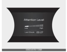
The driver's attention level is displayed on the scale of 1 to 5. The lower the level is, the more inattentive the driver is.
