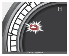
2. When the warning lamp turns ON, the vehicle can drive an additional 20~30 km (12~18 miles) depending on the driving speed, heater / air conditioner, weather, driving style, and other factors. Charging is required.
