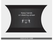
If the driver takes hands off the steering wheel for several seconds while LKA system is activated, the system will warn the driver.
