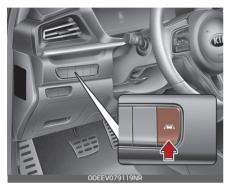
To activate/deactivate LKA system, with the POWER button in the ON position, take the following steps:
