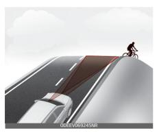
The performance of Forward Collision-Avoidance Assist system may be decreased while driving upward or downward on a slope. The front camera or front radar sensor recognition may not detect the vehicle, pedestrian or cyclist in front.
