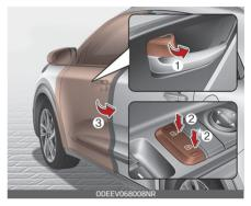
If you lock the door with the central door lock switch (2), all vehicle doors will lock automatically.
