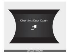
This message is displayed when the vehicle is driven with the charging door opened. Close the charging door and then start driving.
