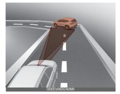
Your vehicle speed can be reduced due to a vehicle in the adjacent lane. Adjust your vehicle speed by depressing the brake pedal according to the road and driving conditions ahead.
