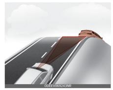
During uphill or downhill driving, Smart Cruise Control system may not immediately detect a moving vehicle in your lane, and may cause your vehicle to accelerate to the set speed.
