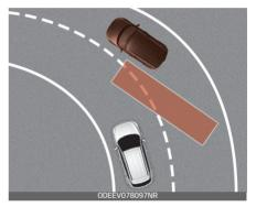
BCW systems may not operate properly when driving on a curved road. In certain instances, the system may not detect the vehicle in the next lane.
