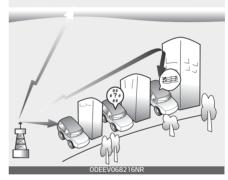
AM and FM radio signals are broadcast from transmitter towers located around your city. They are intercepted by the radio antenna on your vehicle. This signal is then processed by the radio and sent to your vehicle speakers. However, in some cases the signal coming to your vehicle may not be strong and clear.
