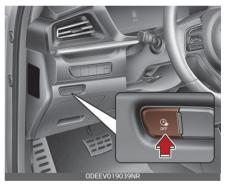
When you press the scheduled charging deactivation button [ for immediate charging, the reserved charge setting is not completely deactivated. If you need to completely deactivate the reserved charge setting, use the multimedia system or the UVO application on your smartphone.
