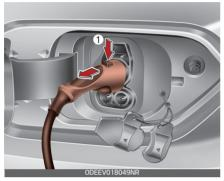
Before disconnecting the charging connector, unlock the vehicle's doors are unlocked. When the doors are locked, the charging connector lock system will be triggered. And the charging connector will not be disconnected. However, in AUTO Mode, the lock is released automatically when charging is completed, and you can disconnect the charging connector.
