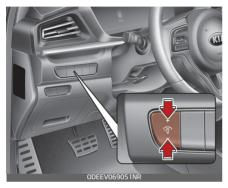
If you hold the illumination control button ("+" or "-"), the brightness will be changed continuously.
