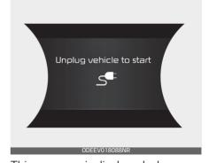
This message is displayed when you start the vehicle, without unplugging the charging cable, and will not shift out of park. Unplug the
