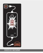
If the charging connector and charging terminal are not connected properly, this may cause a fire.
