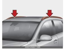
Crossbars and fixing components can be installed on the roof rack to carry cargo. Those may be obtained from an authorized Kia dealer or other qualified shop.
