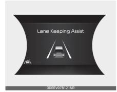
To see the LKA screen on the LCD display in the cluster, Tab to the Driving Assist mode ( ).
