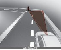
The performance of Forward Collision-Avoidance Assist system may be limited when driving on a curved road.
