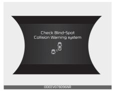
If there is a problem with the BCW system, a warning message will appear and the light on the button will turn off. The system will turn off automatically. Have your vehicle inspected by an authorized Kia dealer.
