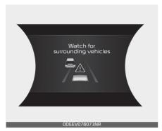
If the vehicle ahead (vehicle speed: less than 30 km/h (20 mph) moves to the next lane, the warning chime will sound and a message will appear. Adjust your vehicle speed for vehicles or objects that can suddenly appear in front of you by depressing the brake pedal according to the road and driving conditions.
