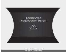
The message will appear when the system is not functioning normally. The system will be cancelled and the word 'AUTO' on the cluster will disappear and instead display regenerative braking level. Check for foreign substances on the front radar. Remove any dirt, snow, or foreign material that could interfere with the radar sensors. If the system still does not operate normally, take
