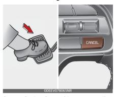
Smart Cruise Control is temporarily canceled when the brake pedal is depressed or the CANCEL button is pressed.
