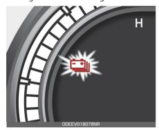
When the warning lamp turns ON the vehicle can drive an additional 20~30 km (12~18 miles) depending on the driving speed, heater/air conditioner, weather, driving style, an other factors. Charging is required.
