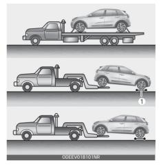
Proper lifting and towing procedures are necessary to prevent damage to the vehicle. The use of dollies (1) or flatbed is recommended.
