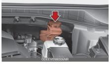
Before removing the reservoir cap and adding brake fluid, clean the area around the reservoir cap thoroughly to prevent brake fluid contamination.
