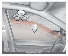
If the window detects the resistance while the power window switch is pulled up continuously, the window will stop upward movement then lower approximately 2.5 cm (1 in).
