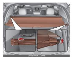
To use the cargo security screen, pull the handle backward and insert the edges into the slots.
