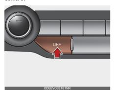
Press the front blower OFF button to turn off the front air climate control system.
