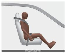
When an adult is seated in the front passenger seat, if the PASSENGER AIR BAG "2" indicator is on, change POWER button to the OFF position and ask the passenger to sit properly (sitting upright with the seatback in an upright position, centered on the seat cushion with their seat belt on, legs comfortably extended and their feet on the floor). Restart the vehicle and have the person remain in that position. This will allow the system to detect the person and to enable the passenger air bag.
