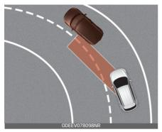
BCW systems may not operate properly when driving on a curved road. In certain instances, the system may recognize a vehicle in the same lane.
