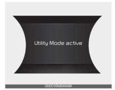
When driving is not necessary such as while camping or when stopping the vehicle for a long time, it is possible to use the electrical devices (audio, lights, etc.) for long hours.
