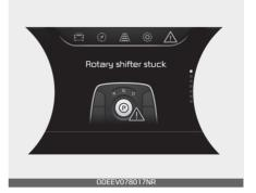
The message appears on the LCD display when the shifter dial is continuously stuck or there is problem with the shifter dial.
