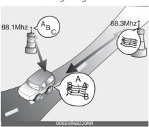
Multi-Path Cancellation - Radio signals being received from several directions can cause distortion or fluttering. This can be caused by a direct and reflected signal from the same station, or by signals from two stations with close frequencies. If this occurs, select another station until the condition has passed.
