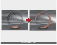
Immediately drive approximately 7~10 km or about 10 min (4~6 miles) to evenly distribute the sealant in the tire. Do not exceed a speed of 80 km/h (50 mph). If possible, do not fall below a speed of 20 km/h (12 mph).
