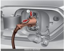
To prevent charging cable theft, the charging connector cannot be disconnected from the inlet when the vehicle's doors are locked. Unlock all doors to disconnect the charging connector from the inlet. However, if the vehicle is in the charging connector AUTO mode, the charging connector automati-
