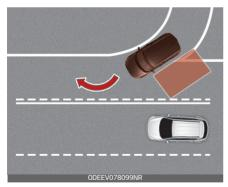
BCW systems may not operate properly when driving where the road is merging/dividing. In certain instances, the system may not detect the vehicle in the next lane.
