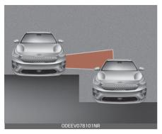
BCW systems may not operate properly when driving where the heights of the lanes are different.
