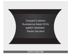
In this case, a warning message ("Forward Collision Avoidance Assist (FCA) system disabled. Radar blocked") will appear to notify the driver. Remove the foreign substances to allow FCA system to function normally.
