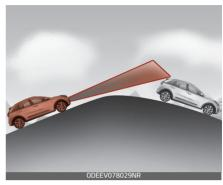
When driving on an uphill or downhill, the system may not detect the vehicle in your lane and the regenerative braking level will reduce automatically, making you feel that the vehicle is accelerating.
