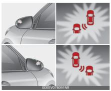
If a vehicle is detected within the boundary of the system, a warning light will illuminate on the outer side view mirror.
