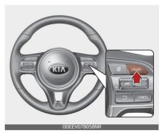
When Smart Cruise Control system is not needed, press the [CRUISE] button and deactivate the system.
