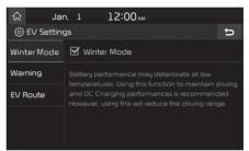
The Winter mode is efficient during the winter time when the high voltage battery temperature is low.
