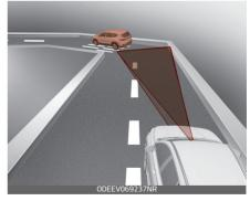
On curves, Smart Cruise Control system may not immediately detect a moving vehicle in your lane, and then your vehicle could accelerate to the set speed. Also, the vehicle
