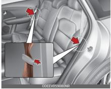
4. Pull on the seatback folding lever, then fold the seat toward the front of the vehicle. When you return the seatback to its upright position, always be sure it has
