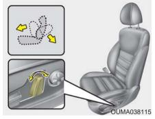
Push the control switch forward or backward to move the seatback to the desired angle. Release the switch once the seat reaches the desired position. Seat height (if equipped)
