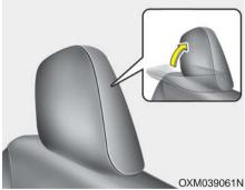
The headrest will fold down automatically when folding the seatback. To fold the headrest manually : Pull the strap.
