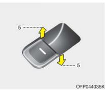
The driver's door has a master power window switch that controls all the windows in the vehicle.
