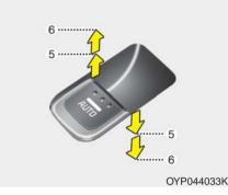
Pressing or pulling up the power window switch momentarily to the second detent position (6) completely lowers or raises the window even when the switch is released. To stop the window at the desired position while the window is in operation, pull up or press down and release the switch.
