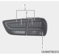
If the stop and tail lamp (LED) (1,2), does not operate, have the vehicle checked by an authorized Kia dealer.
