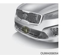
The sensor detects distance to the vehicle ahead.
