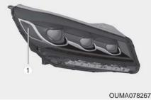
If the side marker (LED) (1) does not operate, have the vehicle checked by an authorized Kia dealer. The LED lamps cannot be replaced as a single unit because it is an integrated unit. The LED lamps has to be replaced with the unit.
