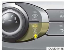
The defroster heats the window to remove frost, fog and thin ice from the rear window, while the engine is running. To activate the rear window defroster, press the rear window defroster button located in the center facia switch panel. The indicator on the rear window defroster button illuminates when the defroster is ON.
