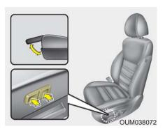
Press the front portion of the switch to raise the cushion extension, or the rear portion of the switch to lower it. Release the switch once the cushion extension reaches the desired position. Seatback angle
