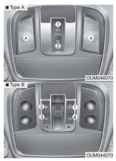
• Press the lens (A) to turn the map lamp on.
