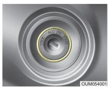
Whenever a front door is opened, the ignition switch will illuminate for your convenience, provided the ignition switch is not in the ON position. The light will go off immediately when the ignition switch is turned on. It will also go off after about 30 seconds when the door is closed.
