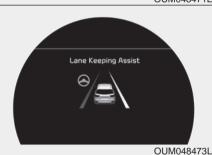
If the vehicle leaves a lane, the lane marker you cross will blink on the LCD display.
