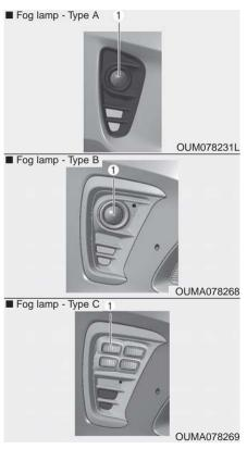
If the front fog lamp (1) does not operate, have the vehicle checked by an authorized Kia dealer.
