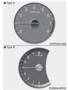
indicates the approximate number of engine revolutions per minute (rpm).
