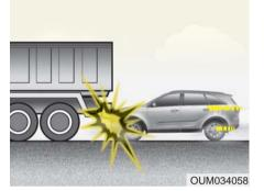
· Just before impact, drivers often brake heavily. Such heavy braking lowers the front portion of the vehicle causing it to "ride" under a vehicle with a higher ground clearance. Air bags may not inflate in this "under-ride" situation because deceleration forces that are detected by sensors may be significantly reduced by such "under-ride" collisions.
