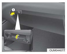
The glove box can be locked and unlocked with a master key. (if equipped) To open the glove box, push the button and the glove box will automatically open. Close the glove box after use.
