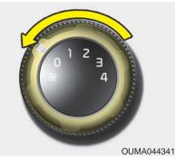
To turn off the blowers, turn the fan speed control knob to the "0" position.
