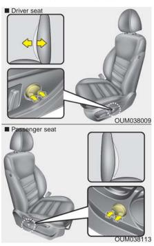
The lumbar support can be adjusted by pressing the lumbar support switch on the side of the seat.
