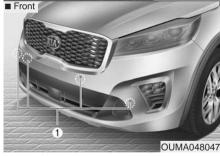
The parking assist system assists the driver during movement of the vehicle by chiming if any object is sensed within the distance of 100 cm (39 in.) in front and 120 cm (47 in.) behind the vehicle. This system is a supplemental system and it is not intended to nor does it replace the need for extreme care and attention of the driver.
