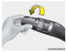
When the light switch is in the parking light position, the tail, license and instrument panel lights will turn ON. Headlight position ( 10)
