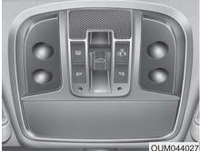
If your vehicle is equipped with a sunroof, you can slide or tilt your suproof with the suproof control lever located on the overhead console
