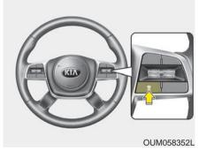
This function allows you to program the vehicle to maintain relative distance to the vehicle ahead without depressing the accelerator pedal or brake pedal. The vehicle to vehicle distance will automatically activate when the smart cruise control system is on.
