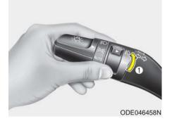
Fog lights are used to provide improved visibility when visibility is poor due to fog, rain or snow, etc. The fog lights will turn on when the fog light switch (1) is turned to the on position after the headlight is turned on.
