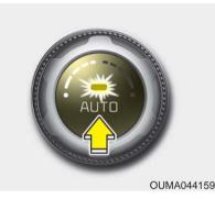
1. Press the AUTO button. The modes, fan speeds, air intake and air-conditioning will be controlled automatically by setting the temperature.
