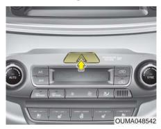
The hazard warning flashers serves as a warning to other drivers to exercise extreme caution when approaching, overtaking, or passing your vehicle. It should be used whenever emergency repairs are being made or when the vehicle is stopped near the edge of a roadway.
