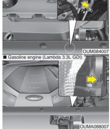
The engine number is stamped on the engine block as shown in the drawing.
