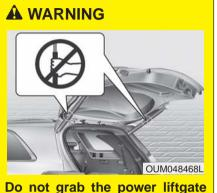
Do not grab the power liftgate struts while the liftgate is open.
