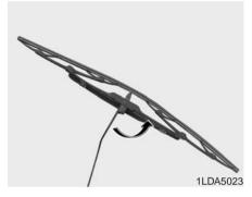
1. Raise the wiper arm and turn the wiper blade assembly to expose the plastic locking clip.
