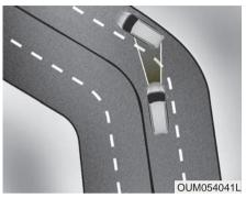
• Your vehicle speed can be reduced due to a vehicle in the adjacent lane. Adjust your vehicle speed by depressing the brake pedal according to the road condition ahead and driving condition. Apply the accelerator pedal and select the appropriate set speed. Check to be sure that the road conditions permit safe operation of the smart cruise control system.
