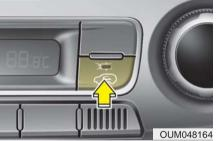
This is used to select the outside (fresh) air position or recirculated air position.
