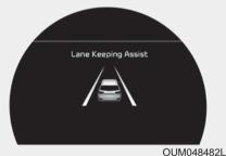
• If the speed of the vehicle is over 64 km/h (40 mph) and the system detects lane markers, the color changes from gray to white. When the conditions below are met, LKA SYSTEM will be enable to assist steering.
