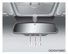
The electric rearview mirror automatically controls the glare from the headlights of the vehicles behind you in nighttime or low light driving conditions. The sensor (4) mounted in the mirror senses the light level around the vehicle, and automatically conrols the headlight glare from the vehicles behind you.
