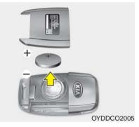
The transmitter uses a 3 volt lithium battery which will normally last for several years. When replacement is necessary, use the following procedure.
