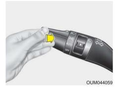
To turn on the high beam headlamp, push the lever away from you. The lever will return to its original position. The high beam indicator will light when the headlight high beams are switched on.
