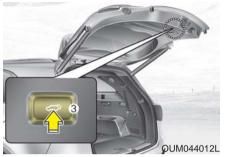
(1) Power liftgate open / close button(2) Power liftgate handle switch(3) Power liftgate close button
