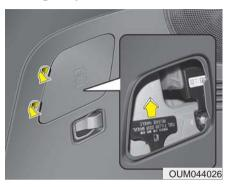
If the fuel filler lid does not open using the remote fuel filler lid release, you can open it manually. Remove the panel in the cargo area. Pull the handle out slightly.
