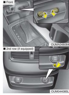
The power outlet is designed to provide power for mobile telephones or other devices designed to operate with vehicle electrical systems. The devices should draw less than 10 amps with the engine running.
