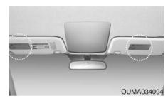
Air bag warning labels, some required by the Canada Motor Vehicle Safety Standards (CMVSS), are attached to the sunvisor to alert the driver and passengers of potential risks of the air bag system.
