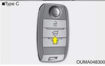
• Press the power liftgate close button for approximately one second when the liftgate is opened.
