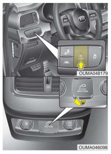
The AC inverter supplies 115V/150W electric power to operate electric accessories or equipment.
