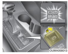
To apply the EPB (electronic parking brake):
