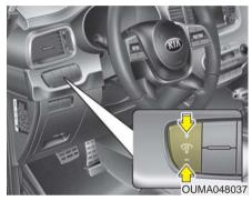
The brightness of the instrument panel illumination is changed by pressing the illumination control button ("+" or "-") when the ignition switch or Engine Start/Stop button is ON, or the tale lights are turned on.
