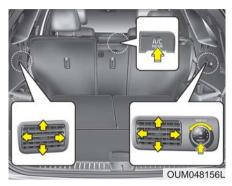
To turn on the third row air conditioning control system 1. You can operate the third row air conditioning system from the first row control panel. Changing the front row's fan speed by pressing the control button will automatically change the third row's fan speed as well.
