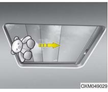
If an object or part of the body is detected while the sunroof is closing automatically, it will reverse the direction, and then stop.
