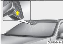
The Lane Keeping Assist System detects the lane markers on the road with a front view camera at the front windshield, and assists the driver's steering to help keep the vehicle in the lanes. When the system detects the vehicle straying from its lane, it alerts the driver with a visual and audible warning, while applying a slight countersteering torque, trying to prevent the vehicle from moving out of its lane.
