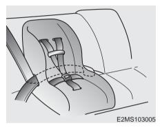
The auto lock mode will help prevent the normal movement of the child in the vehicle from causing the seat belt to loosen and compromise the child restraint system. To secure a child restraint system, use the following procedure.
