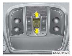
*To open the sunshade* Pull the sunroof control lever backward to the 1st detent position.
