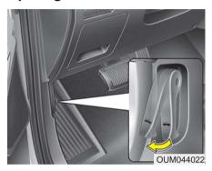
1. Pull the release lever to unlatch the hood. The hood should pop open slightly.
